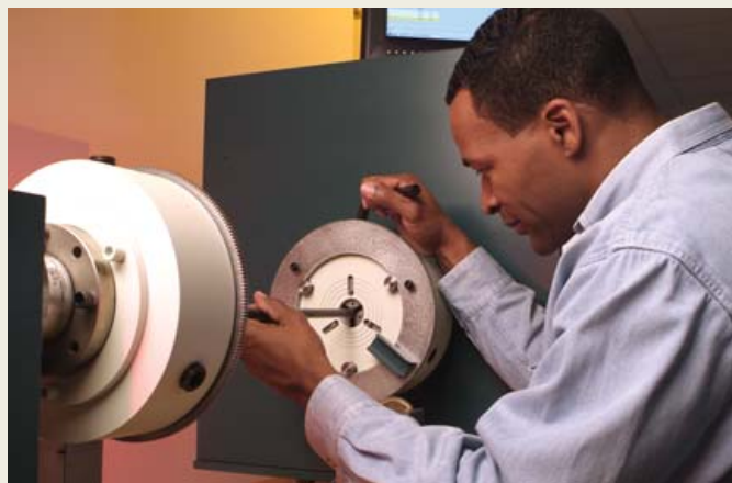
Fig 6. Samples are easily mounted in the patented bi-directional grips.
