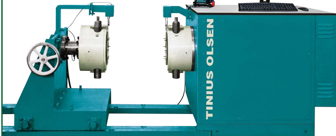
Fig 1. 200,000 in.lbf torsion tester for testing samples that are up to 7 ft long and 5 in diameter (2.1 m long and 125 mm diameter). The machine is shown with the optional PC based software.
