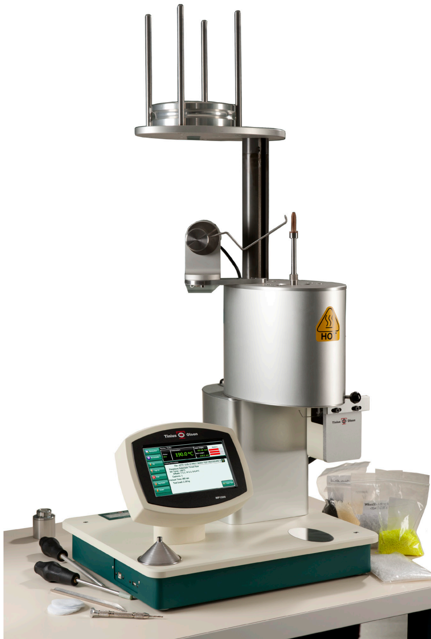
Fig 4. Motorized MP1200 shown with Programmable Piston Displacement Transducer and Automatic Cutter.
