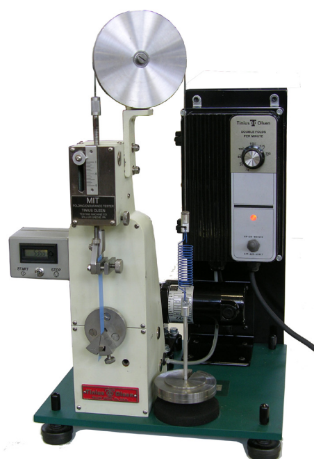
Fig 2. Model 2 Folding Endurance Tester with modified loading system, digital counter and variable speed drive is for use on materials with relatively high amounts of elongation.
