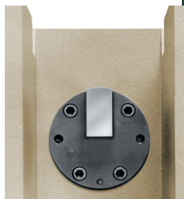
Fig. 8. View of the Izod striker from the pendulum head.
