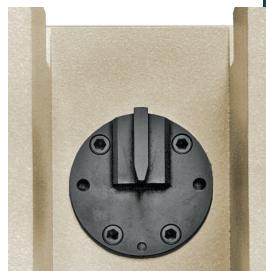
Fig. 6. View of the Charpy striker from the pendulum head.
