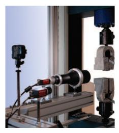
**Figure 3.** Dual camera setup, one camera with materials testing lens and the other camera with a general purpose lens; also showing mounting bracket and light source (if required).
