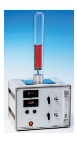
ASTM D 2863: Standard test method for measuring the minimum oxygen concentration to support candle-like combustion of plastics (oxygen index)
